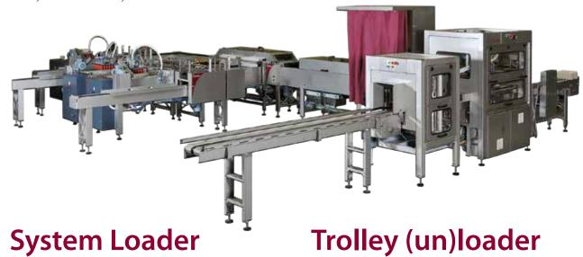
The System Loader carefully feeds eggs from their transport tray to the Setter Line modules like the proven PSPC setting
